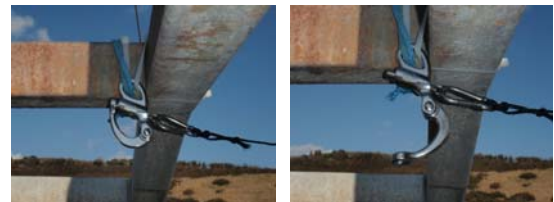
Figure 10: End weight quick release system
