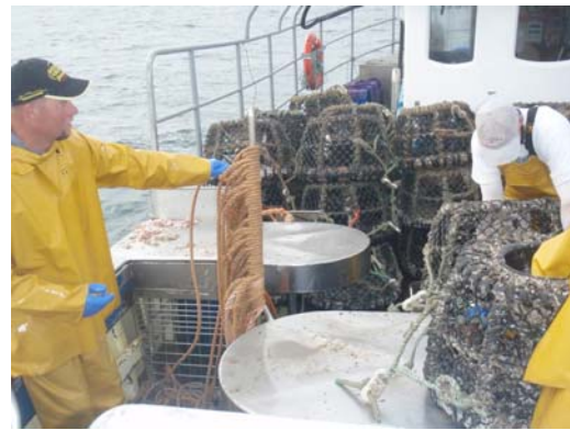
Figure 2: Placing the eye splice on the pole ready for shooting.
