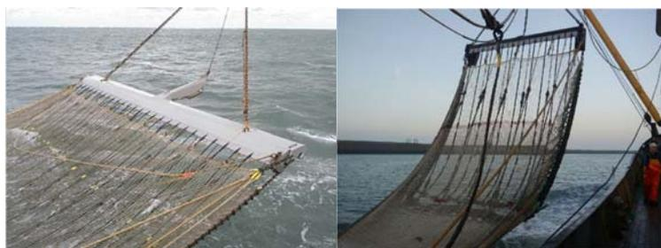
Figure 2 HFK Sum Wing with pulse trawl (left) and Delmecco trawl (right).
