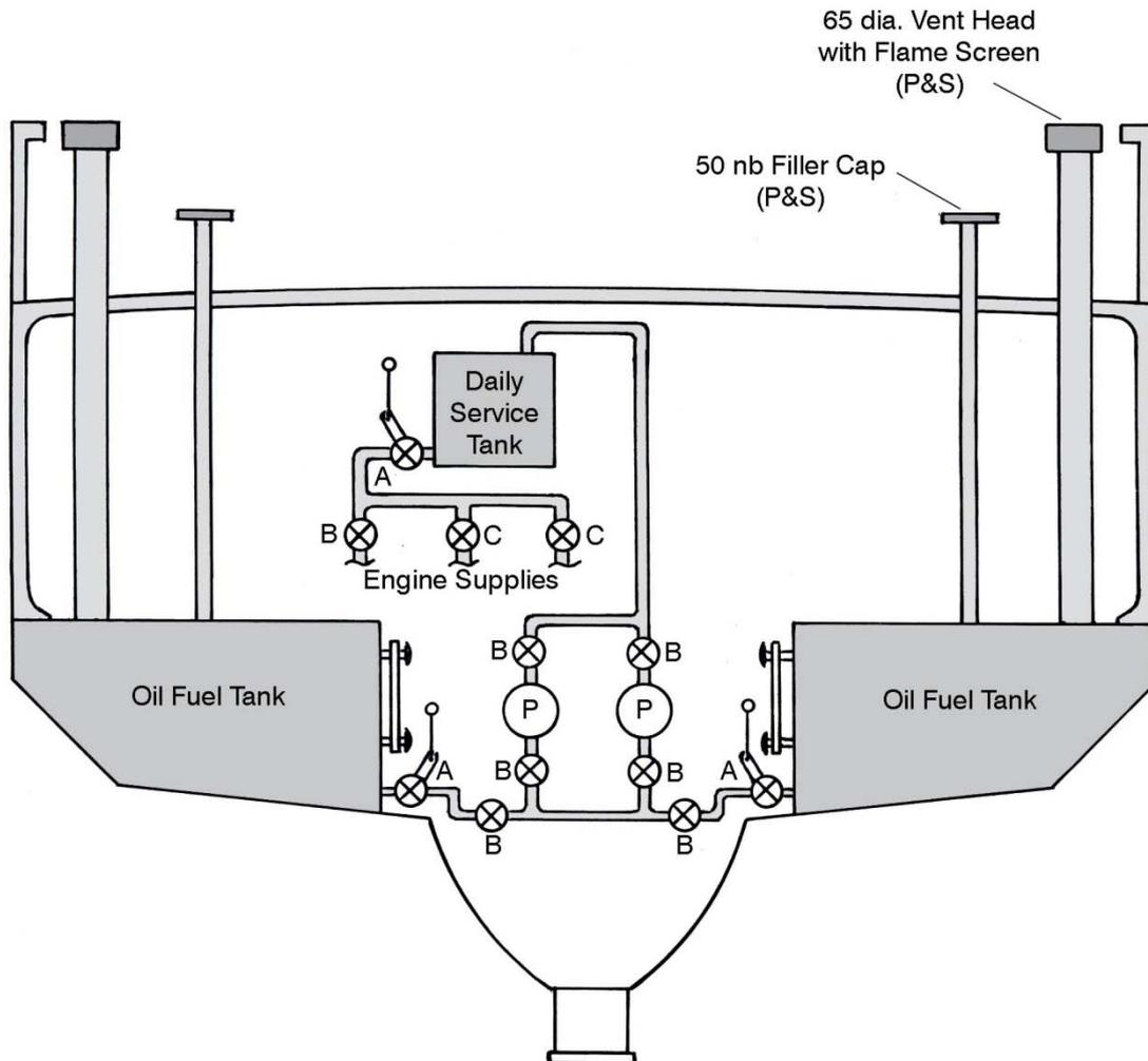
A = 25 nb Tank Ball Valve for Trip Wire
