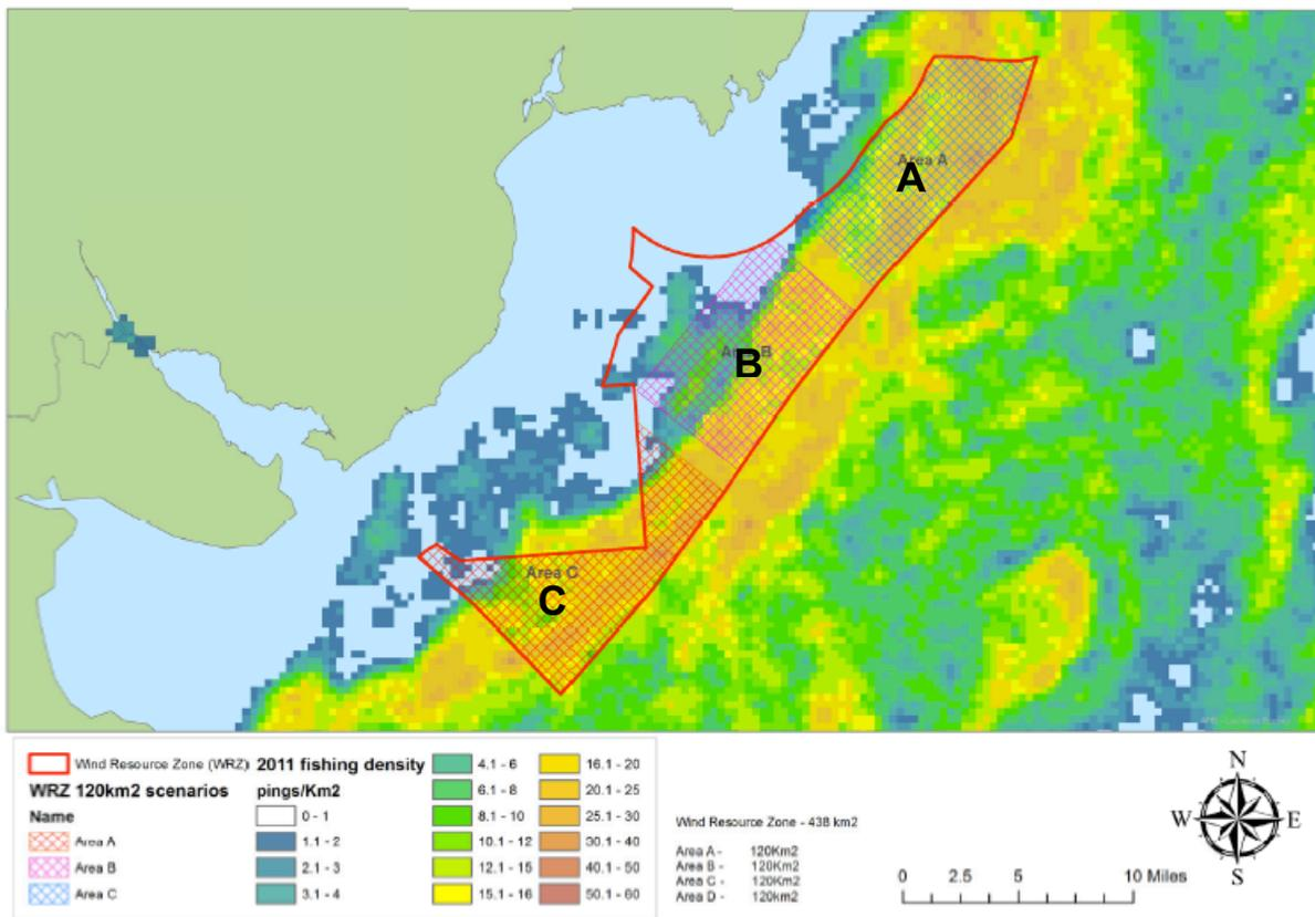
**Figure 1 Wind Resource Zone (red) and potential wind farm development areas (A, B & C), each 120km<sup>2</sup>**
