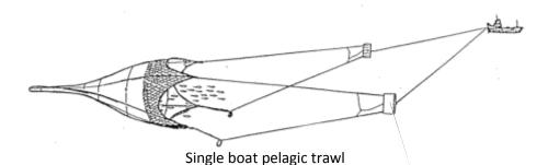
The nets in both methods are handled exactly the same as bottom trawls except that the larger pelagic boats usually pump their fish aboard in the same manner as purse seiners rather than lifting the full cod end aboard. Some of the larger vessels are capable of catching several hundred tons in one haul.
