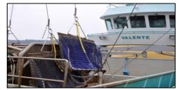
Figure 18. Valente with mussel dredge equipment (© R. Whiteley)
