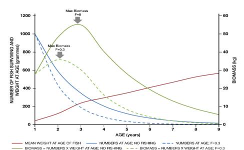
Figure 2; The calculation of the biomass of a cohort of 1000 fish with an age of first capture of age 1 over the time it passes through the stock. The red line is the growth in weight with age of individual fish in grams, the blue lines are the number of fish surviving with age and the green lines are the number of fish surviving multiplied by the weight at age showing how the biomass of the cohort varies with age (the dashed lines represent a fishing mortality of F=0.3).
