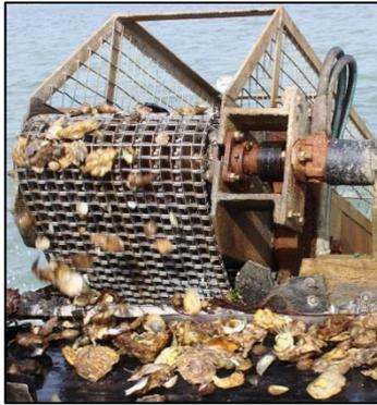
**Figure 24. Shellfish harvester used by Othniel Oysters in Poole Harbour**
