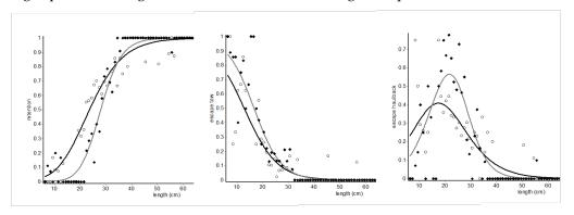
Fig. 7. Results for cod for T0 (black curve) and T90 (grey curve): overall codend retention (left), escape during towing (middle), escape during haulback operation (right).
