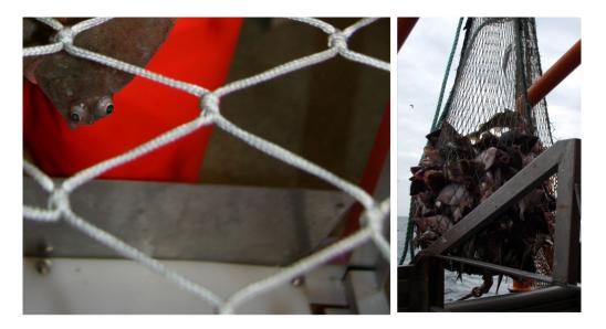
Fig. 3. Dyneema single 2.5 twine and codend (right) applied during the cruise.
