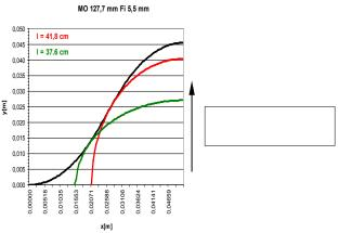
Fig. 12. Length that cod can escape from a T90 codend (black is the deformed T90 mesh bar and red ("Vertical" position of cod) or green ("Horizontal" position of cod) the cross section of the fish).
