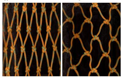
Fig. 1. Polytit COMPACT (redline) applied for the codends.
