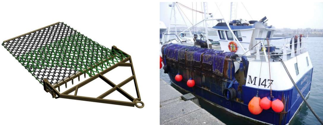
*Figure 2 Scallop dredge, left; and scallop dredging vessel, right (source: Seafish)*
