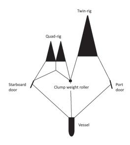
Figure 1. Trial gear rigging
