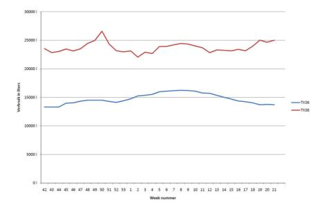
Again the red line is from the TX38 witch now uses the normal SumWing. Fuel saving for the TX36 in this period is 260.000ltr.
