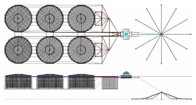
**Figure 25** Canadian Aquaculture Engineering Group (AEG – Canada). Above – plan view of six cages attached to framework and through a feed and service barge to a single point mooring system. Below – side view of system (http://www.aquacultureengineeringgroup.com).
