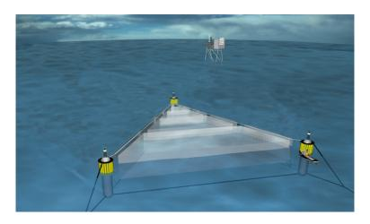
**Figure 32** Diagram of one segment of the conceptual MFRL design. This enclosure system would be by far the largest single cage unit if deployed (courtesy of Maris Fish Ranches Ltd.)
