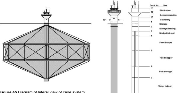
**Figure 45** Diagram of lateral view of cage system and detail of central spar of the conceptual Ocean Drifter cage.
