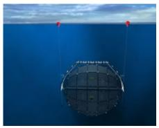
Figure 42 Position 4: Extremesubmerged, this position occurs in extreme situations like algae invasions, unfavourable temperatures, storms/typhoons etc. or if the breaded fish naturally belongs in the deep water
