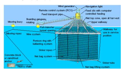
**Figure 27** Diagram of Farmocean cage showing complete system in side view (http://www.farmocean.se).
