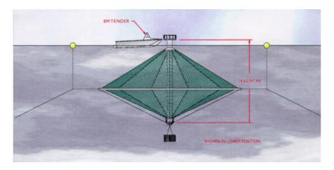
**Figure 34** Diagram of Oceanspar cage submerged (see - http://www.masgc.org/oac/gallery01.html and http://www.oceanspar.com/pictures.htm)
