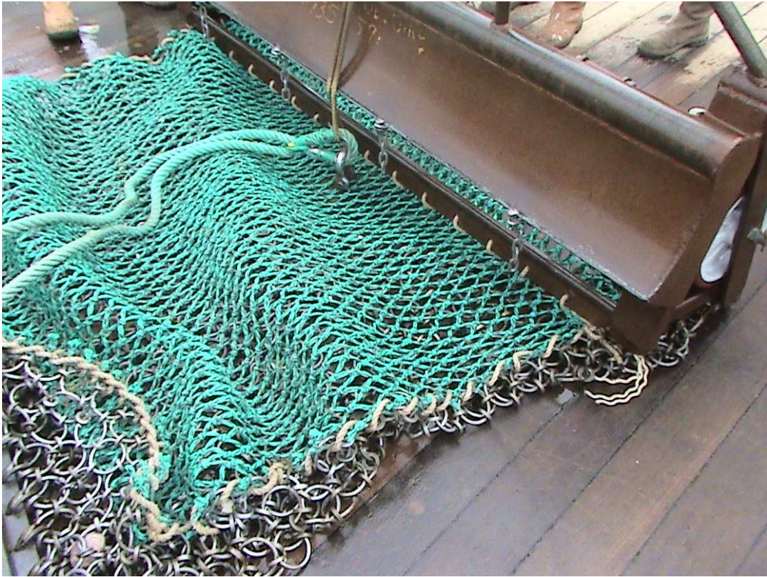
Figure 2. Experimental bag fitted to the hydrodredge during preliminary trials.
