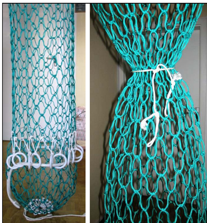
Figure 3. Model of T90 codend (1:3)
