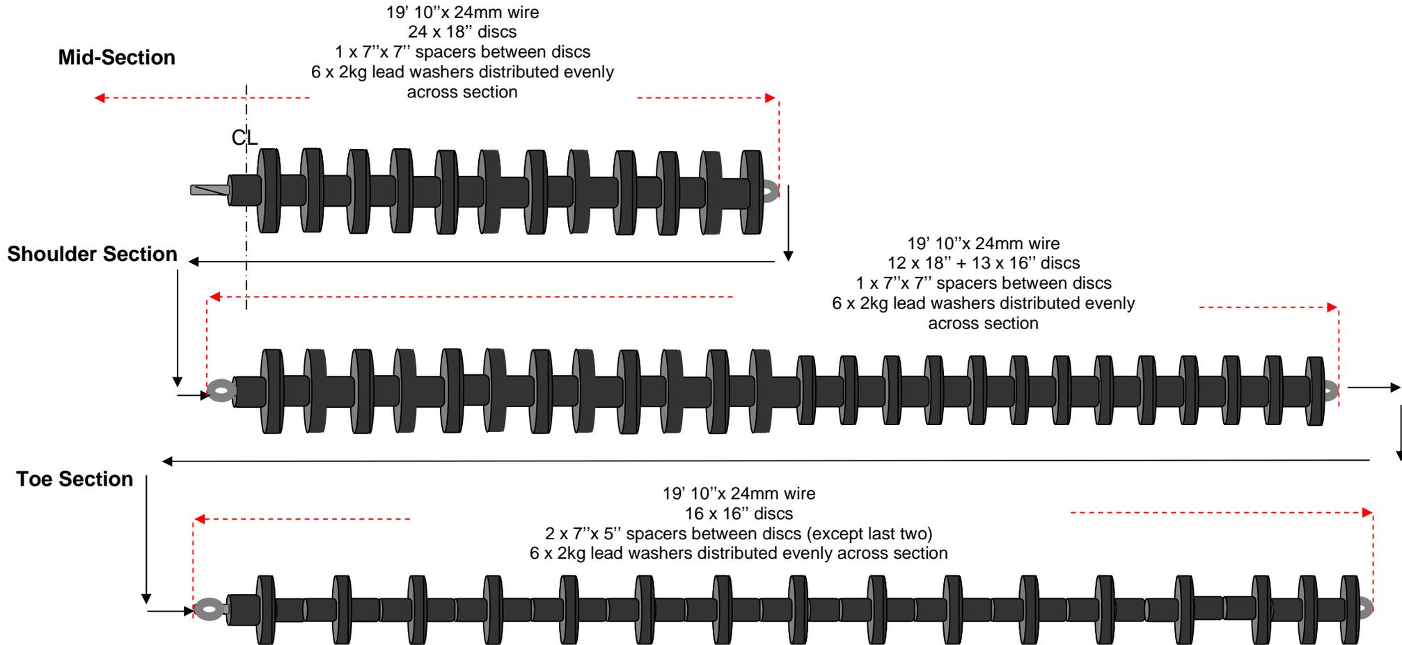
Figure (3): Outline schematic showing relative shape and size of trawls under test
