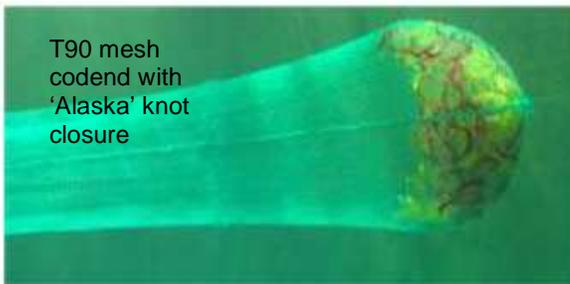
Images of model codends in the Flume Tank showing the relative shapes and potential influence on catches.
