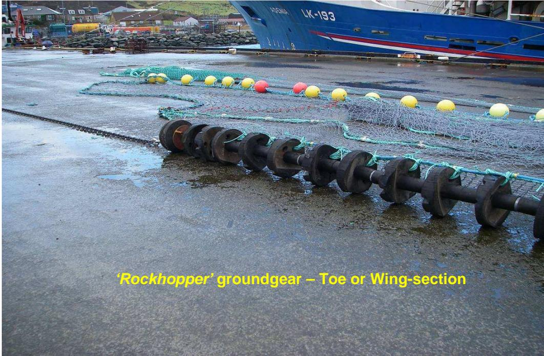
The *toe-end* of the groundgear was finished off with a *'bumper-bobbin'* arrangement forming the connection to the groundgear extension chains (2 x ~10.5m x 16mm mid-link) via a 12" *'bouncer pin'*. (See photos for details).
