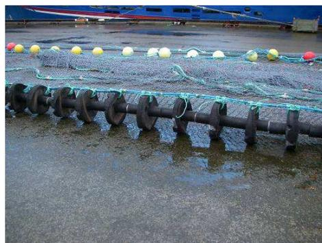
The mid-section consisted of 1 x 19'10" (~6.0m) length of 24mm wire with 24 x 18" (457mm) rubber 'Rockhopper' discs. The discs were separated by 1 x 7" x 7" (178mm x 178mm) rubber spacers. Extra weight in the form of 6 x 2kg lead washers was evenly distributed over the length of the centre section.
