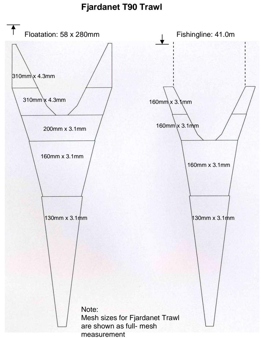
Figure (4): Codend arrangements for the standard and T90 trawls
