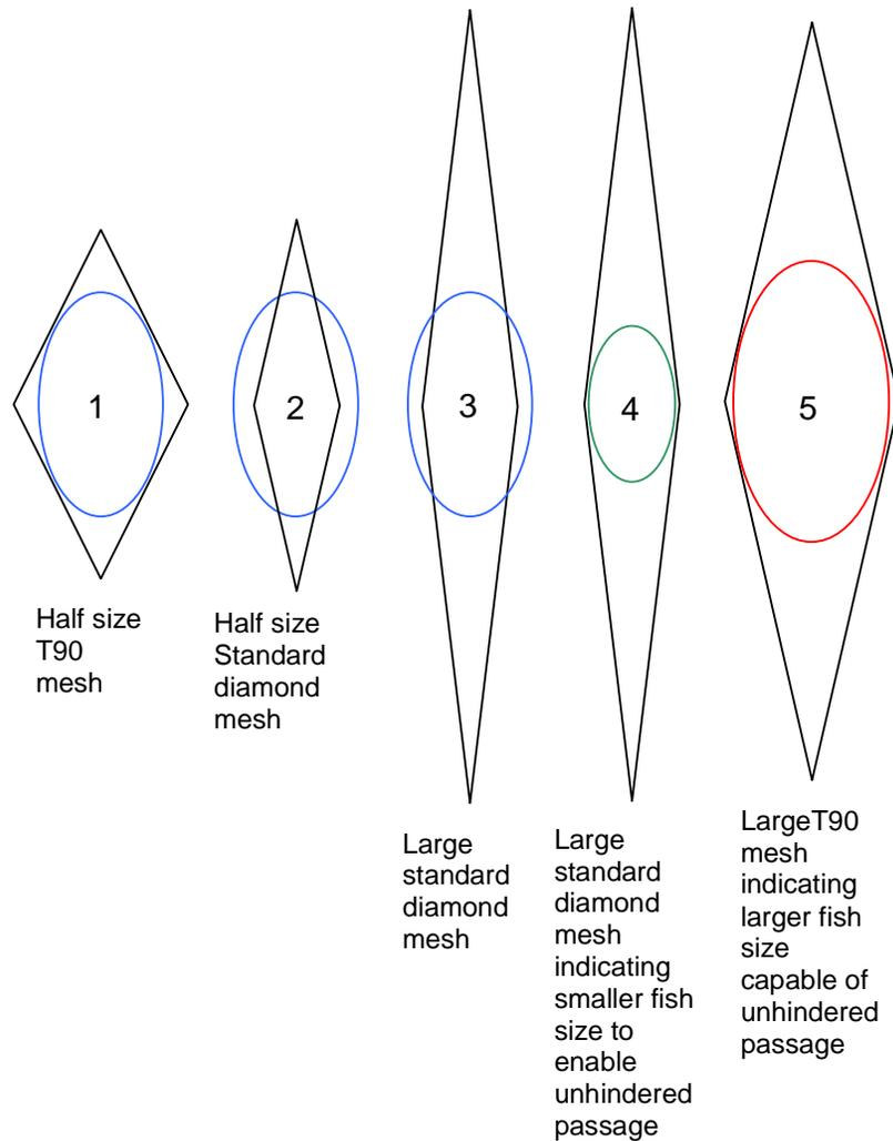
It is possible for a fish of a given size to pass through T90 mesh of a mesh size compatible with its body shape and size without incurring injury/damage caused by forces exerted on the fish by the mesh bars (1)
