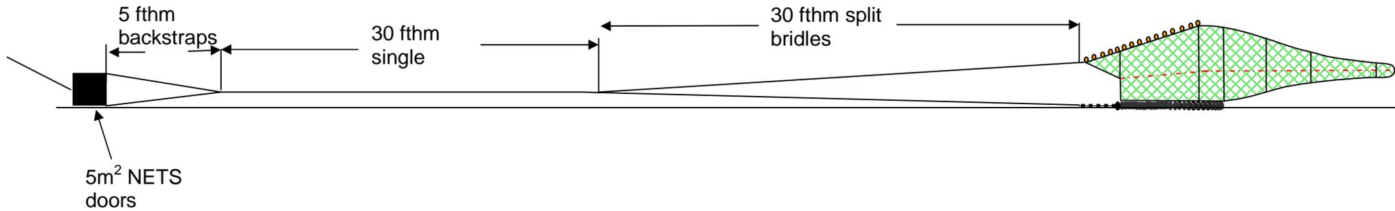
Figure (2): **Ground Gear specification – ‘Rockhopper’ rig**
