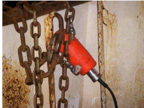
SCANMAR load cell measuring tension behind the trawl doors
