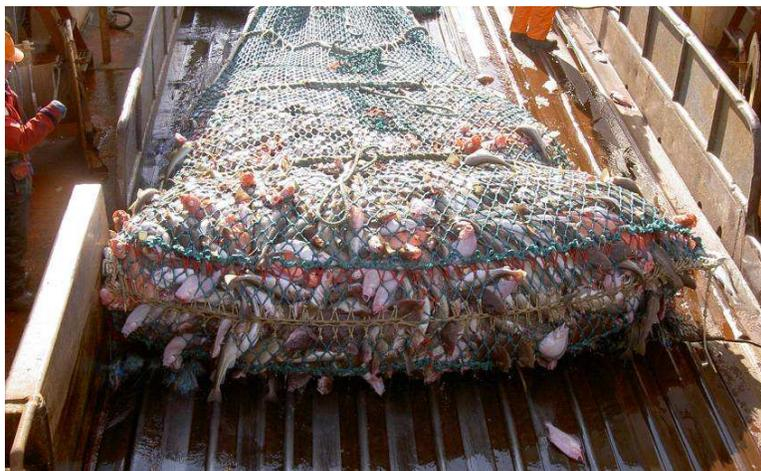
T90 codends with catch onboard Icelandic vessel
