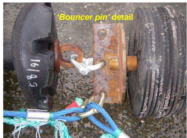
The groundgear was attached to the fishingline of the net using 8mm, 3-strand PP/PE rope fastened through the top hole of the 'Rockhopper' discs.
