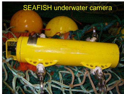
The underwater camera was used on a limited number of tows when and where conditions were suitable. Due to poor water clarity it was difficult to obtain much useful film of the gear. Some images of the mouth of the trawl were obtained giving an indication of the net rigging on the fishingline and groundgear and showing consistent mesh opening achieved by the T90 netting.
