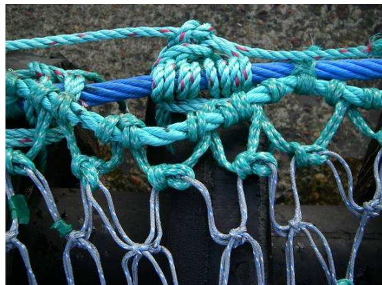
**Crown meshes in belly panel showing bolsh attachment to fishingline**
