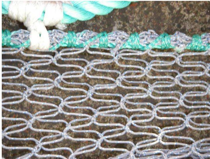
**Section of a T90 extension showing consistent mesh opening**
