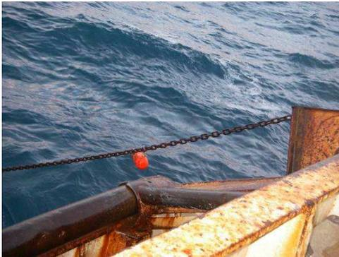
SCANMAR distance sensor on trawl door
