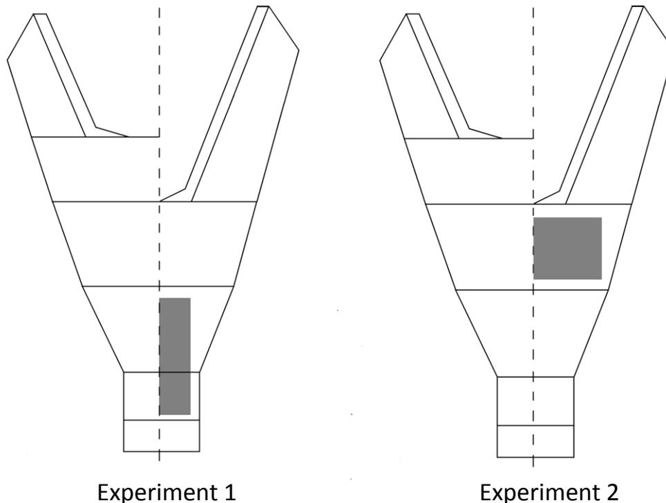
Figure 3 The two positions tested for the square-mesh panel on the underside of the trawl.
