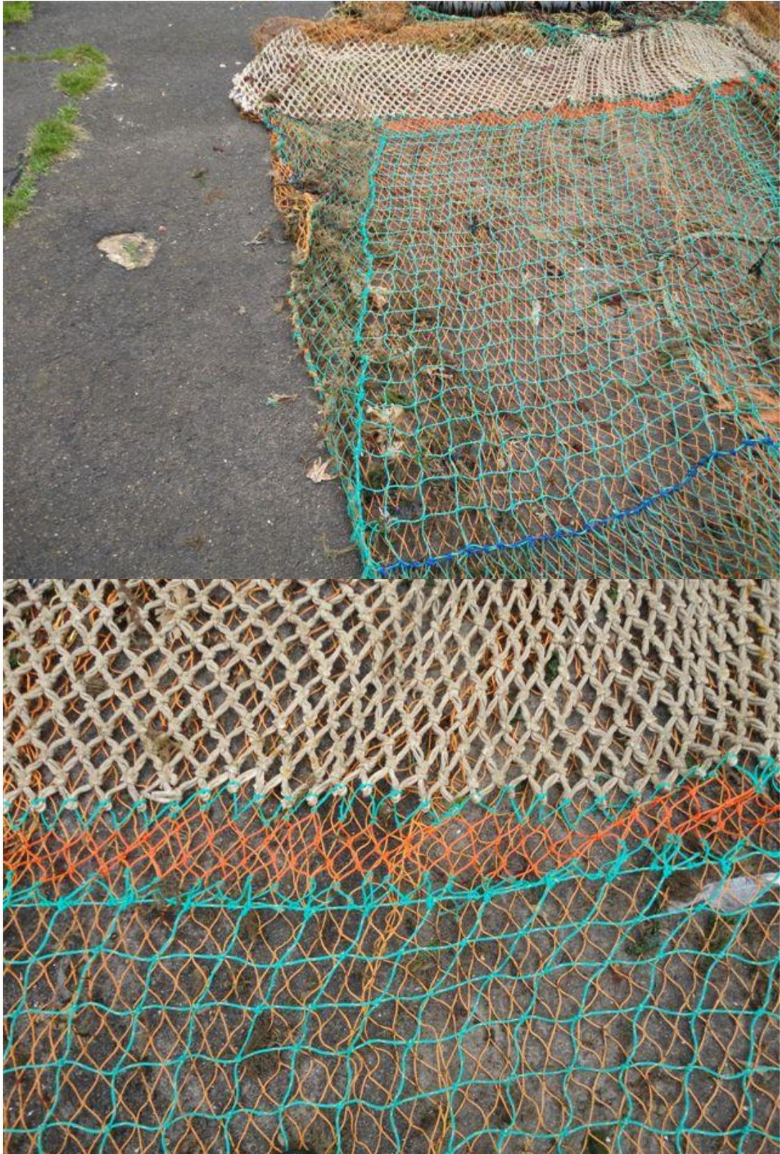
Figure 5 Position and fitting of the square-mesh panel for experiment 2, constructed of 120 mm diamond-mesh PPE
