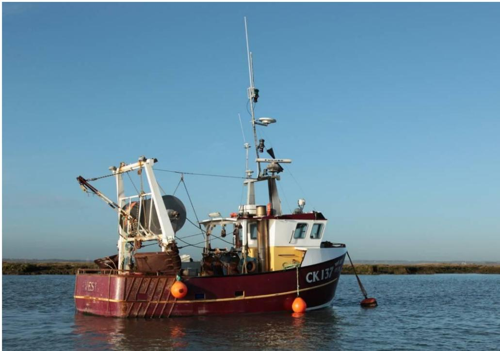
Figure 2 MFV “Harvester”, LOA 9.96 m, GT 16.08 t, main engine 112 kW
