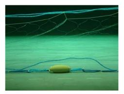
Figure 1 Pingers in flume tank; left AIRMAR Pinger attached next to a float, right AQUAmark pinger attached to tangle net leadline.
