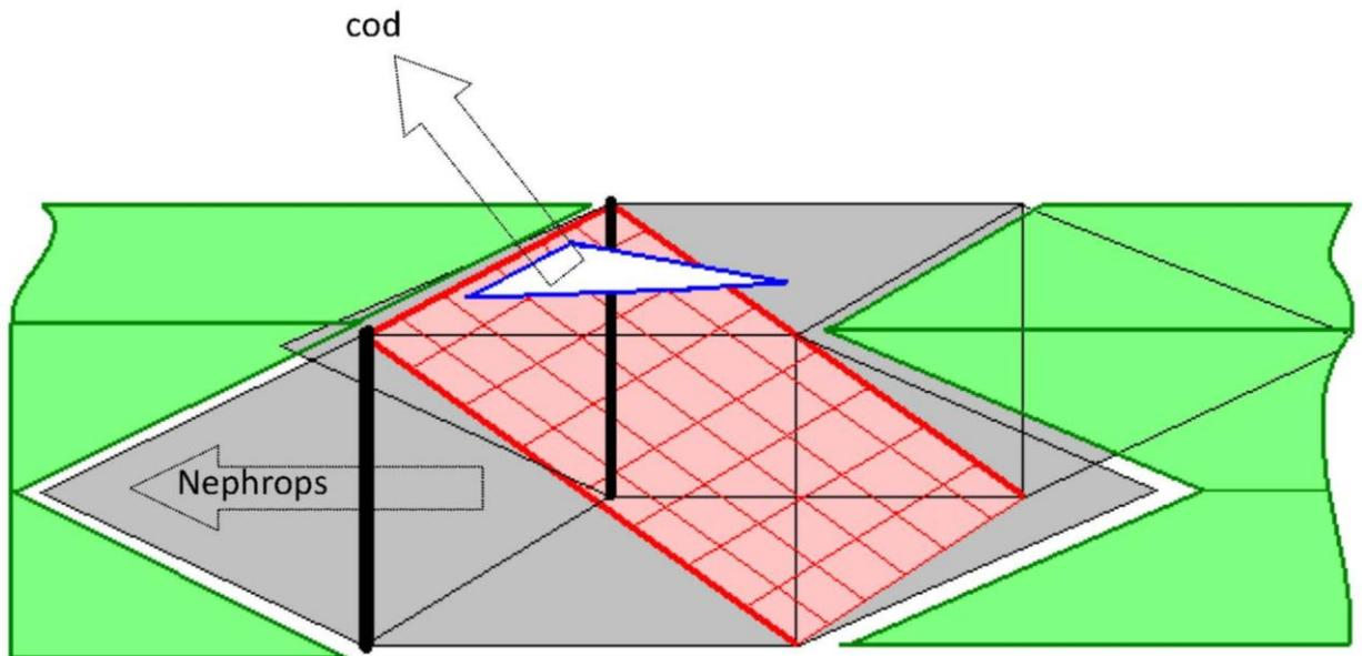
Figure 3 Plan of Net Grid with cutting ratios for the insertion of the box section and fish escape hole
