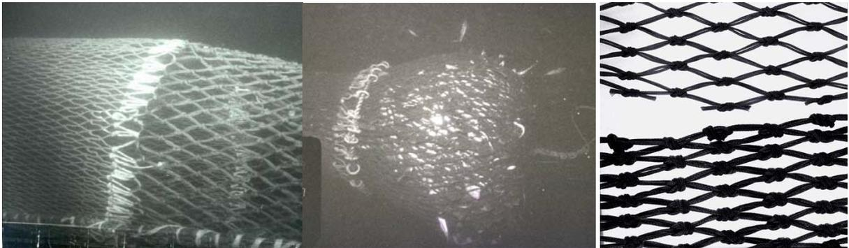
**Figures 5c-5e:** Left - Narrow codend with fewer meshes around circumference attached to standard extension showing increased mesh opening. Centre - Lifting bag of double the mesh size on the outside of codend. Right - Two samples of netting with similar sized mesh but different twine thickness.
