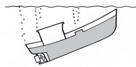
If the boat has no watertight bulkheads and if the bilge pump cannot cope with the leak, the boat will certainly sink.
