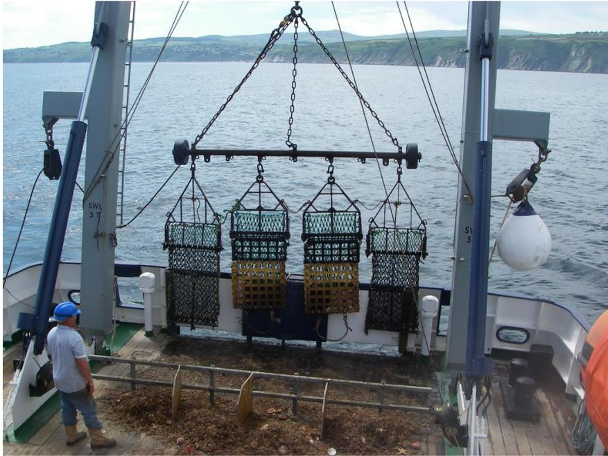
Figure 6: Sea trials of the Oban dredge (centre two dredges) against standard Newhaven dredges (outer two dredges). Source: Bill Lart, Seafish.
