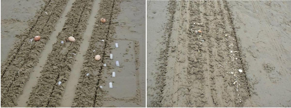
Figure 9: Beach experiment demonstrating the much reduced impact on eggs and shells of a dredge with skids (left) than without skids (right). Images: H. Hinz.
