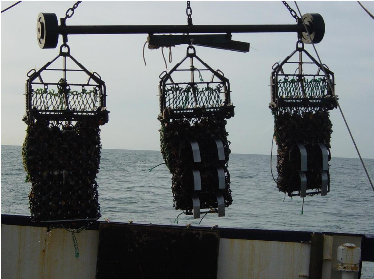
**Figure 8:** Image of dredges with (from right to left) two and three skids attached, during sea trials. Designed by Ewout Costerus (Cyclone Marine Ltd) and John Coppack (Gannet Marine Ltd). Image: Ewout Costerus.
