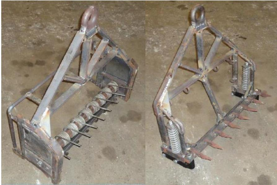
Figure 5: The N-Virodredge design (left) separate from the steel belly bag, with individually sprung tines and side skirts; compared to the Newhaven dredge (right) with a fixed tooth bar. Source: Filippi, 2013.
