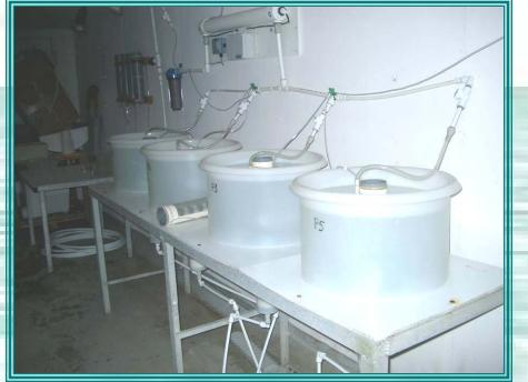
Typical 70 L "Paxton" conical vessels, suitable for cod egg incubation
