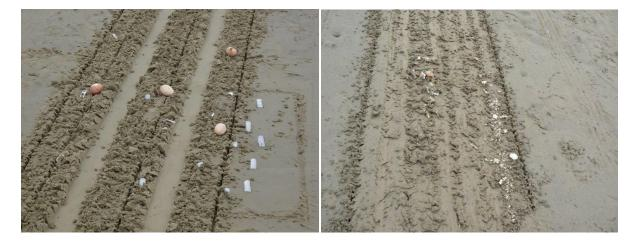
Figure 9: Beach experiment demonstrating the much reduced impact on eggs and shells of a dredge with skids (left) than without skids (right). Images: H. Hinz.
