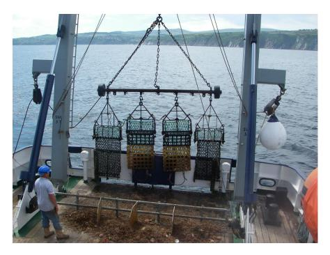
Figure 6: Sea trials of the Oban dredge (centre two dredges) against standard Newhaven dredges (outer two dredges). Source: Bill Lart, Seafish.
