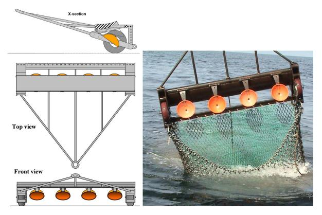
Figure 7: Diagram and image of the Hydrodredge, showing the four rubber cups that replace the tooth bar. Source: Shephard *et al.*, 2009.
