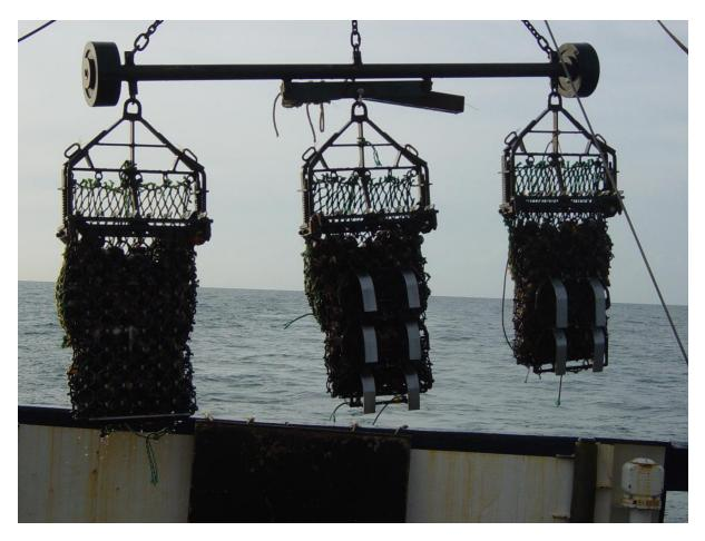
Figure 8: Image of dredges with (from right to left) two and three skids attached, during sea trials. Designed by Ewout Costerus (Cyclone Marine Ltd) and John Coppack (Gannet Marine Ltd). Image: Ewout Costerus.
