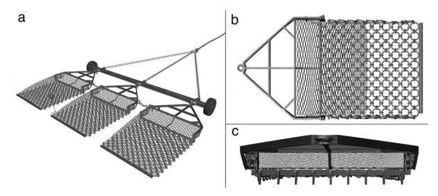
Figure 3: Newhaven king scallop dredge design: (a) aerial view of a gang of 3 dredges attached to the tow bar; (b) top elevation of the steel rings of the belly bag; (c) forward elevation of the tooth bar. From Boulcott & Howell, 2011.
