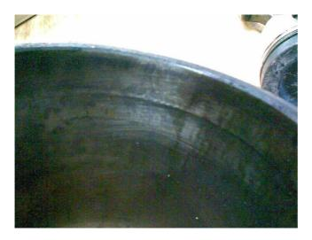
Figure 1Excessive wear: ring landing area
