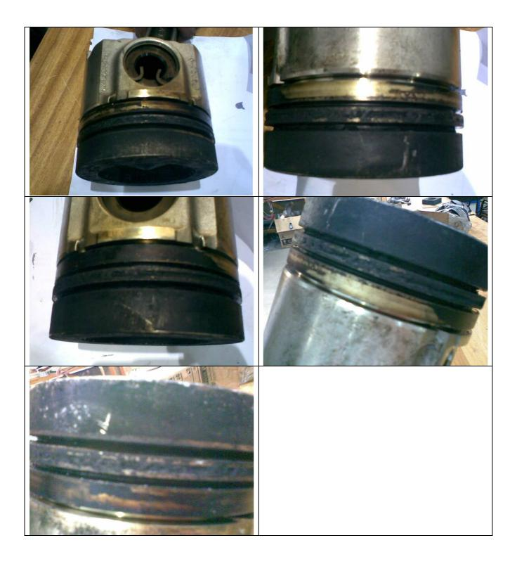
Figure 3 Fingerprints for excessive blow by- possibly due to excessive wear of rings and liner at the ring landing area, hard carbon build-up between top and bottom ring
