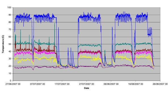
— ambient — Diesel DST — main tank — generator lift pump — generator injection pump — engine injection pump
