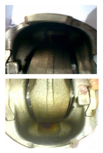
Figure 5 Fingerprint for Overheating: under the piston crown
