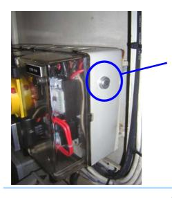
Temperature data logger fixed to switch box in engine room to capture ambient temperature (4). ALL loggers have been set to capture the temperature at 90 minute intervals. Each logger will hold approximately 25 days worth of data.
