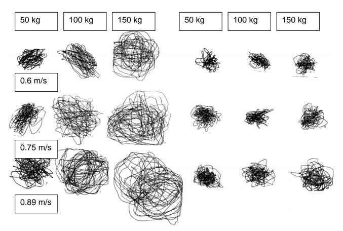
Figure 3 Recordings of codend movements as a function of speed (horizontal) and catch size (vertical). 9 at left: Standard 2 selvedge outside, 9 at right: T90
