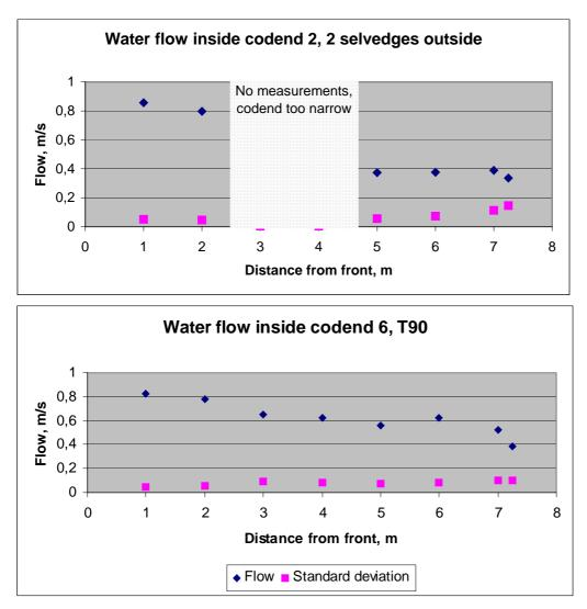
**Diagram 1 Flow measurements in 2 codends**
