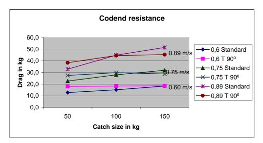
Diagram 2 The relation between catch size and drag in two different codends (no. 2 and 6) at 3 different towing speeds.
