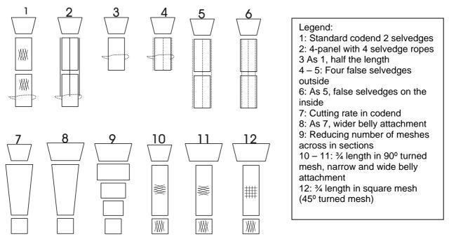
Figure 1 Draft specifications of 12 different codend designs tested in half scale in Flume Tank
