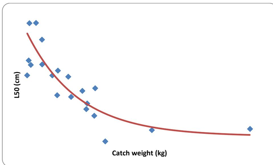
Fig. 11. L50 for cod vs codend catch weight for T90 codend applied during norwegian experimental fishing. The marks represent experimental results for individual hauls while the curve represents the fit of formula (1) to the data applying the method described in Fryer (1991).
