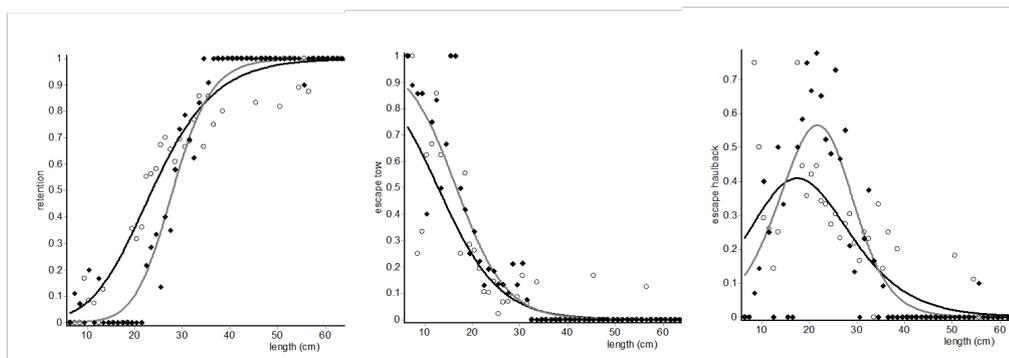
Fig. 7. Results for cod for T0 (black curve) and T90 (grey curve): overall codend retention (left), escape during towing (middle), escape during haulback operation (right).
