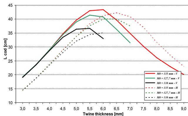
Fig. 13. Calculated length of cod vs. twine thickness for T90 codends.
