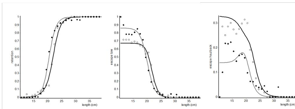
Fig. 8. Results for Plaice for T0 (black curve) and T90 (grey curve): overall codend retention (left), escape during towing (middle), escape during haulback operation (right).
