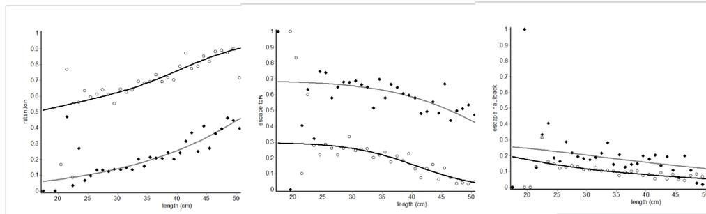
Fig. 9. Results for Nephrops for T0 (black curve) and T90 (grey curve): overall codend retention (left), escape during towing (middle), escape during haulback operation (right).
