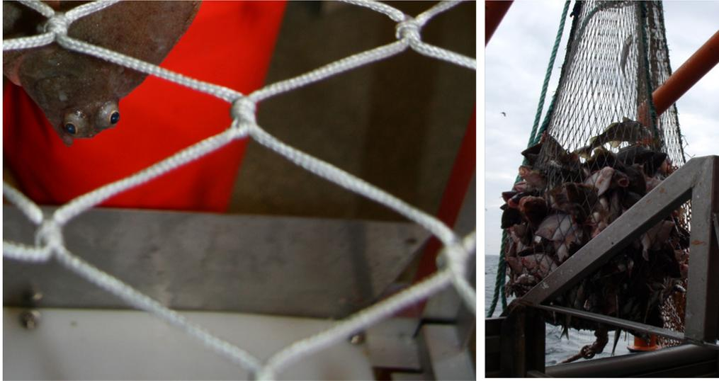
Fig. 3. Dyneema single 2.5 twine and codend (right) applied during the cruise.
