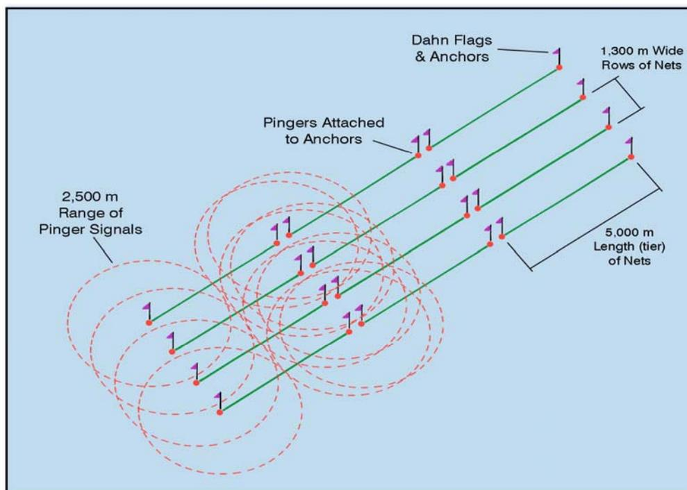
**Figure 5 Possible configuration of large scale pingers**
