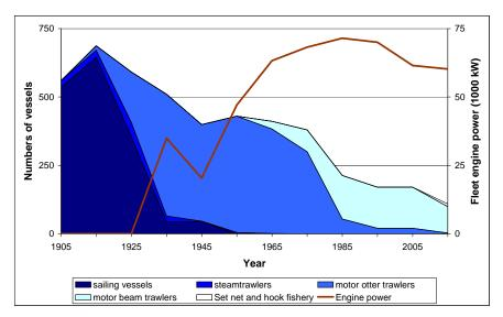
FIG. 2 – HISTORIC EVOLUTION OF THE BELGIAN FISHING FLEET IN NO.'S OF VESSELS BY VESSEL TYPE AND BY TOTAL FLEET ENGINE POWER (POLET ET AL., 1998)
