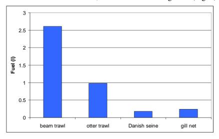
FIG. 5 - FUEL CONSUMPTION IN LITERS FOR 1 KG OF FISH (THRANE, 2004)
