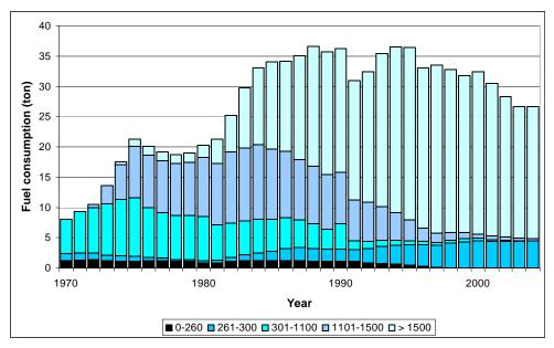
FIG. 4 - TOTAL FUEL CONSUMPTION OF THE BEAM TRAWLER FLEET BY ENGINE POWER CLASS (SMIT AND BUISMA, 2006).
