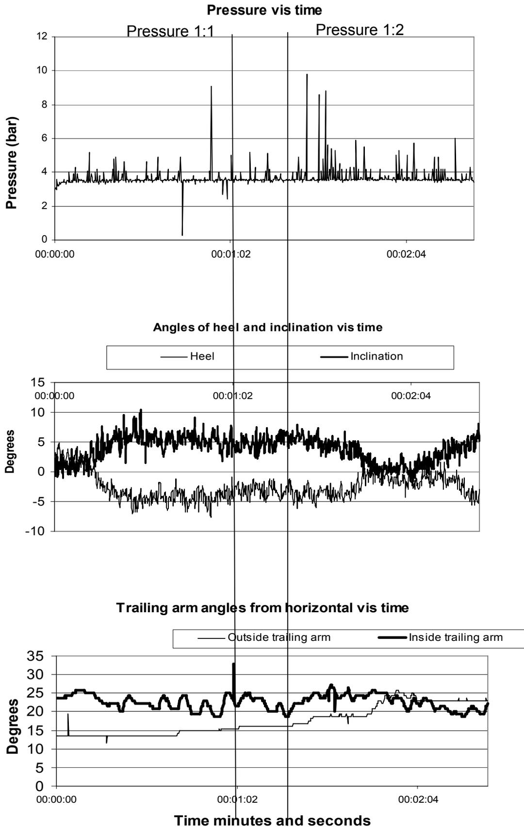
Figure 3.10 Instrumentation Data from haul on Sunk Sand site. Vertical lines correspond to stages in Table 3.5 and Figures 3.15 and 3.16
