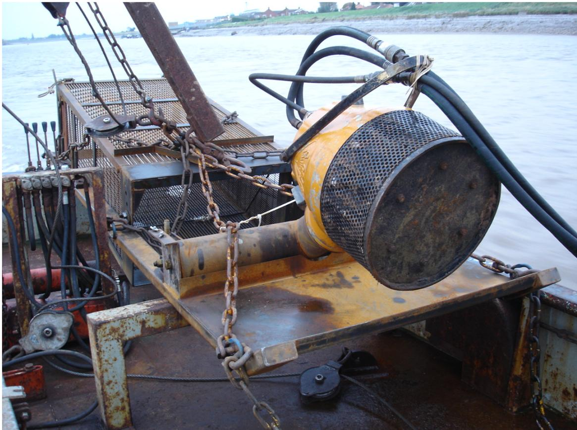
Figure 3.3 Hydrainer 150-D25 pump with high head impeller bolted to experimental dredge
