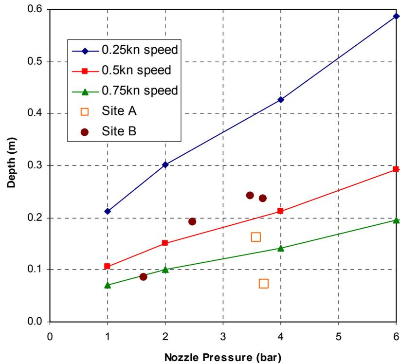
Figure 7 : Depth of Fluidisation – Trial Data and Theoretical Results.
