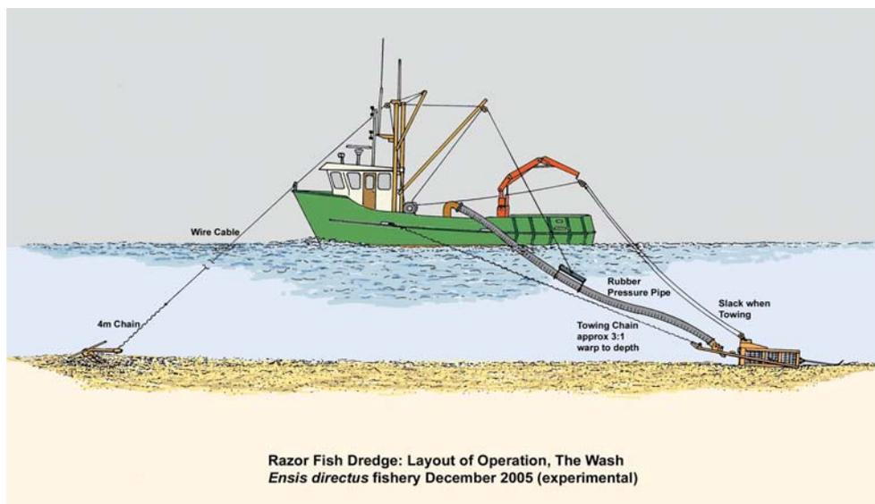
Sixty six metres (36 fathoms of wire) were hauled at the rate required. The distance covered was determined by the odometer reading on the GPS. This usually corresponded to 50-55m of distance over the ground dependent on the degree of slack in the system. The actual speed was computed from the time and distance travelled. The dredge was then hauled back alongside and placed on the aft deck using the HIAB crane. The catch was swept out of the back of the dredge using a broom via the rear door.
