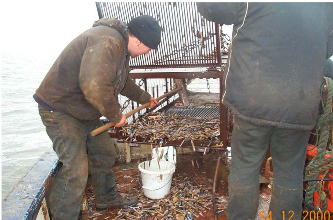
Figure 3.1. b Emptying the catch of razorfish following deployment of the experimental dredge
