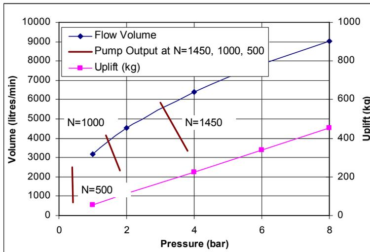
Figure 3.5 Pump curve for the Etanorm 125-315 pump
