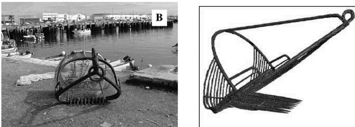
Although optimised for other bivalve species (Gaspar, 2003), the key commercial limitations of this type of dredge are the high level of breakage and damage to *Ensis spp.* inflicted during fishing and the high level of grit and sand remaining in the razorfish after fishing which may preclude them from being sold to the live market without a viable method of de-gritting or depuration.
