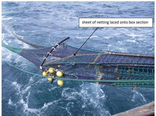
Figure 2 Conceptual diagram of the Net Grid, Nephrops pass through a sheet of netting which is laced into a four panel box section to the codend, while cod and other fish are guided to the escape hole.
