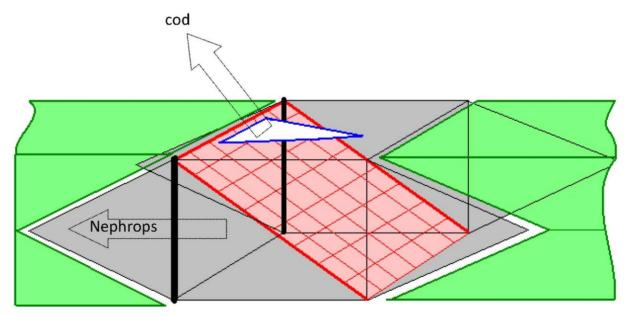
Figure 3 Plan of Net Grid with cutting ratios for the insertion of the box section and fish escape hole
