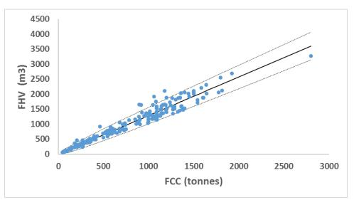
Figure 2. Relationship between FHV (m<sup>3</sup>) and FCC (tonnes) and 95% confidence intervals.
