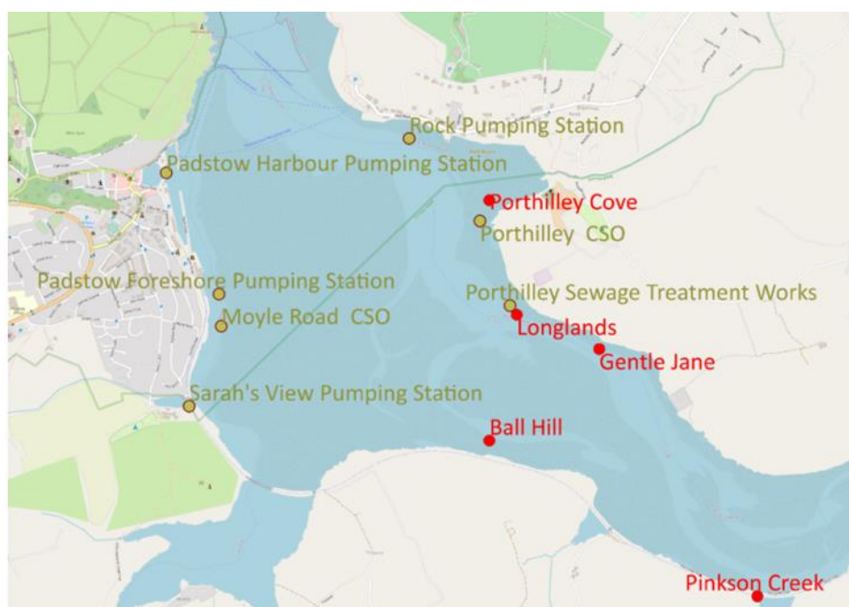
Figure 6.5.5. Location of combined sewage overflows and pumping stations (in green) close to shellfish beds (in red) in the Camel estuary.
