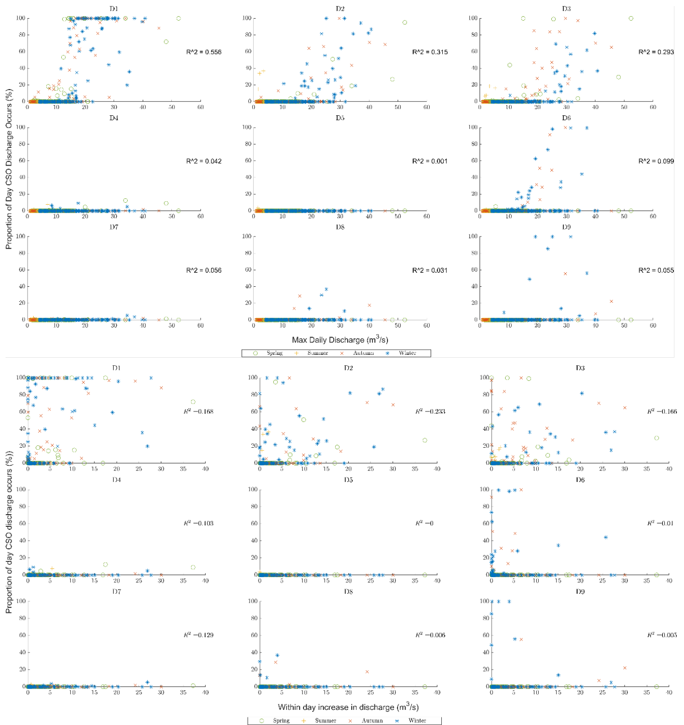
Figure 3.5 Scatter plots of the proportion of days that each CSO discharge on any given day against (top) the maximum river discharge on that day ( Q_{dmax} ) and (bottom) the within day increase in river discharge ( Q_{dinc} ), i.e., the overall increase in river discharge that occurred on each day from the daily min flow to the daily maximum flow where the daily minimum flow was always taken as the minimum flow proceeding the maximum flow; where the maximum river flow occurred at the beginning of the day the within day increase was recorded as zero. Circles are coloured by season. D1-D9 are locations of intermittent discharges given in Table 3.1
