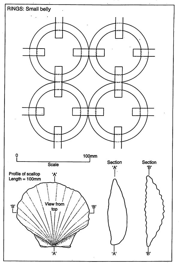
Figure 31: - Ring profile compared with Scallop profile - small belly
