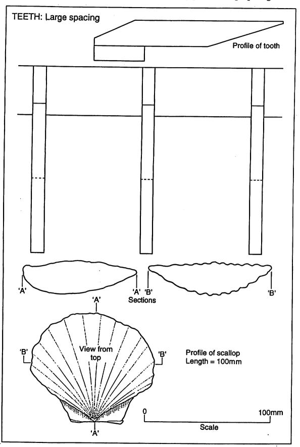
Figure 36: Tooth profile compared with Scallop profile - large spacing
