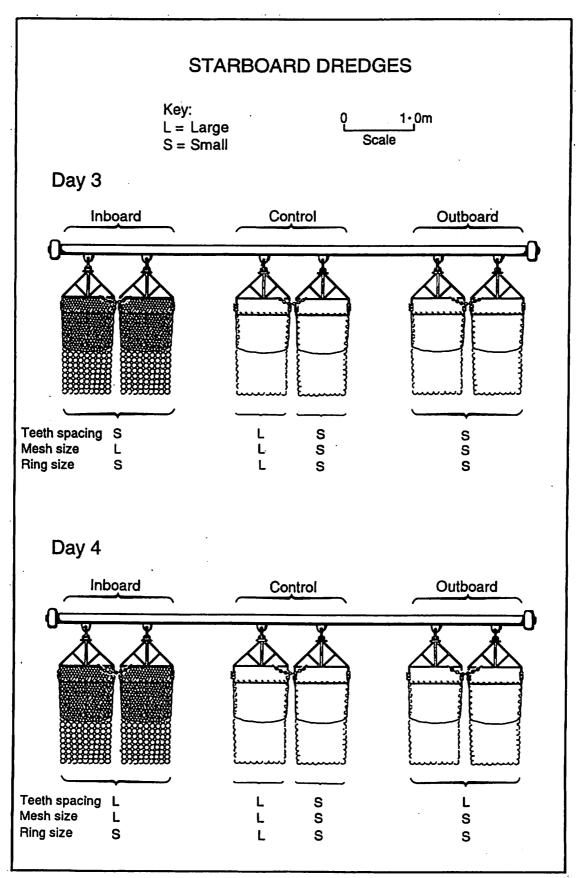
Figure 9: Dredge configurations - days 3 and 4
