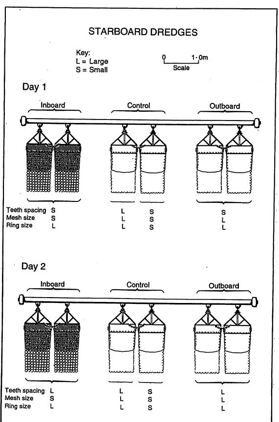
Figure 7: Dredge configurations - days 1 and 2
