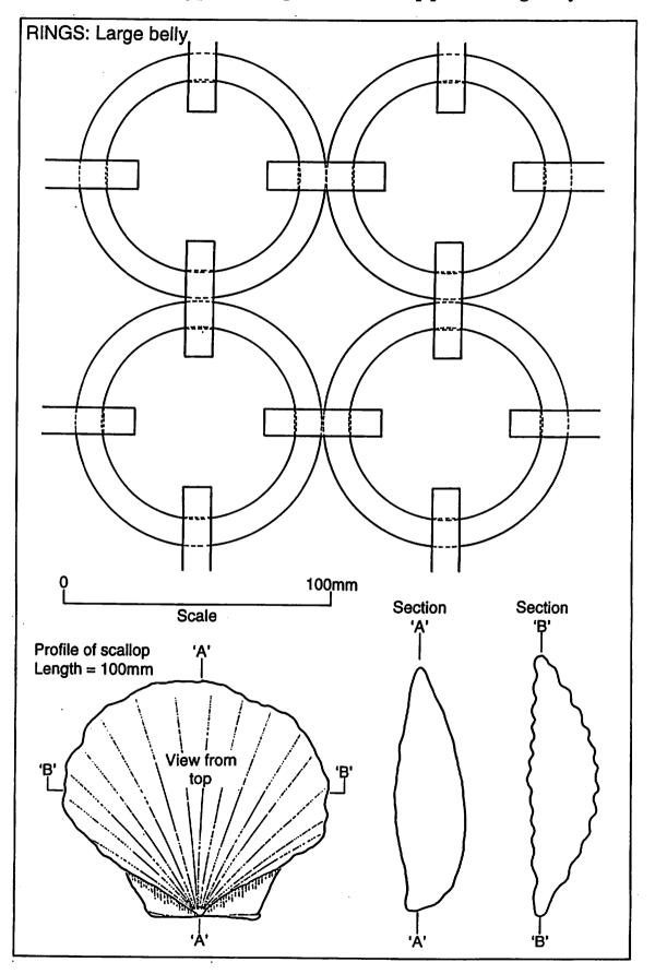
Figure 32: Ring profile compared with Scallop profile – large belly
