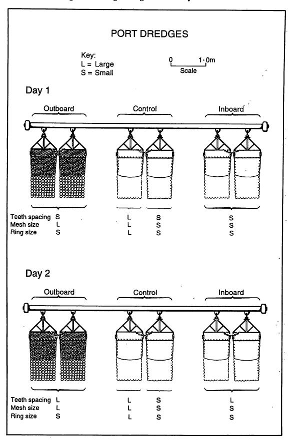
Figure 6: Dredge configurations - days 1 and 2
