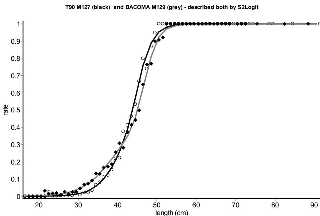
Fig. 5. Average size selection for new T90 codend (black curve) and new BACOMA codend (grey curve).
