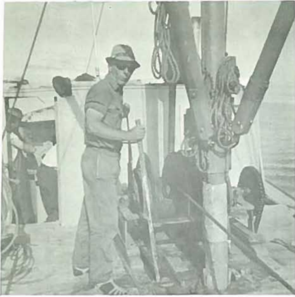
Winch after modification to drums.
