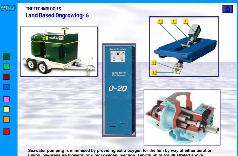
(using low-pressure blowers) or direct oxygen injection. Typical units are illustrated above.
