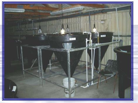
Typical 450 L fibreglass conical vessels, suitable for halibut egg incubation
