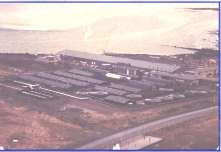
Another marine fin fish land based ongrowing unit, using a combination of circular and rectangular tanks, 0.8 m deep. All tanks have light-shading covers to prevent UV damage. Seawater is pumped on to the farm via submersible pumps at sea, coming into the header tanks on the left of the picture. It is then distributed by gravity to the main farm, via a network of PVC pipes.
