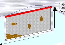
Cage floor pulled upwards by surface motion of this part of flotation collar
