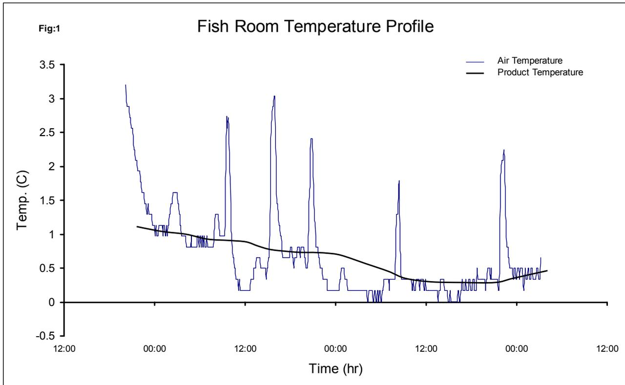
The above temperature profile illustrates how air temperature in the refrigerated hold of a vessel will fluctuate rapidly due to continuous hatch opening during fishing operations. The temperature of the catch, which has already cooled primarily due to action of the ice melt-water, remains relatively stable.
