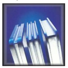
To make good fish blocks you need strong straight frames to hold the fish block liner or fish block carton in the correct shape during freezing in a plate freezer. The photo above shows three different aluminium freezing frame profiles. Left to right they are the "XU" (strongest), the "E" and the "U" (less strong). Most modern processing factories and vessels use the "XU" for its strength and longevity.
