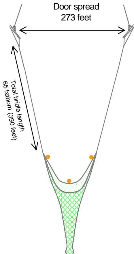
The skipper's target door spread is 60% of his total bridle length. 60% of 390 feet is 234 feet.
