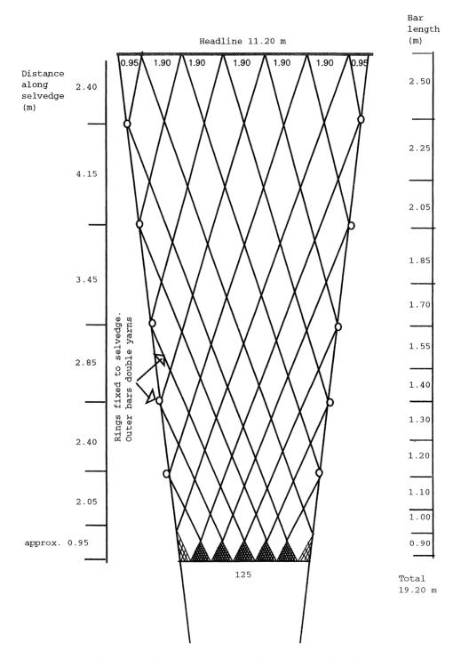
Fig. 4. Large diamond mesh top panel, 12 m version trip 1, 3 and 7.
