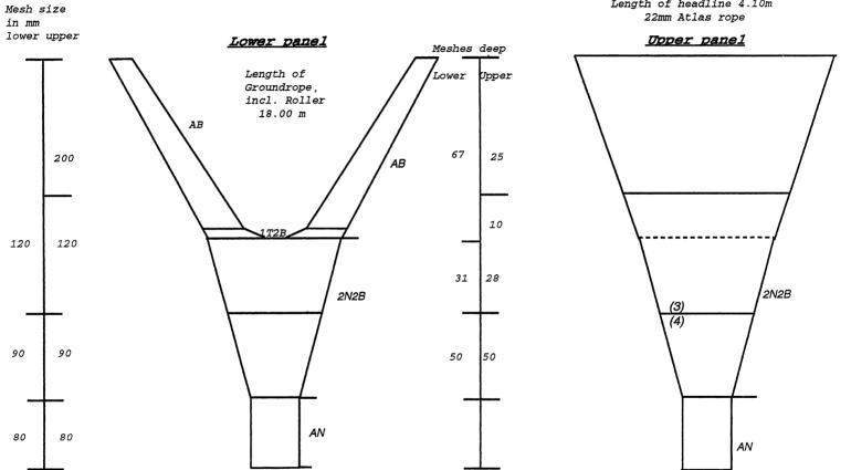
Fig. 2. Net plan conventional beam trawl used on trip 4-6.
