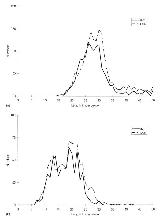
Fig. 7. (a) Length frequency distribution of cod catches (300 hp vessel); (b) length frequency distribution of whiting catches (300 hp vessel); (c) length frequency distribution of cod catches (1500–2000 hp vessels); (d) length frequency distribution of whiting catches (1500–2000 hp vessels); LMT: large mesh top panel; CON: conventional gear.
