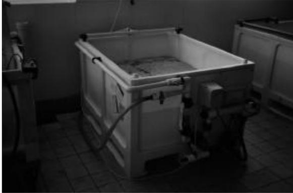
This system has been developed for mussels only, as they remain active in deeper layers than most molluscs. The mussels are held in a 350mm deep layer in a number of specially modified plastic pallet bins. Each bin is transportable and is connected to a common seawater supply and return system.
