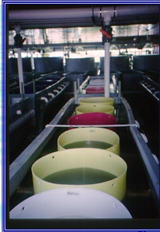
Water circulates from the reservoir upwards through the mesh on the base of each upwelling cylinder. Flow rate is controlled by a valve at the outlet of each cylinder.
