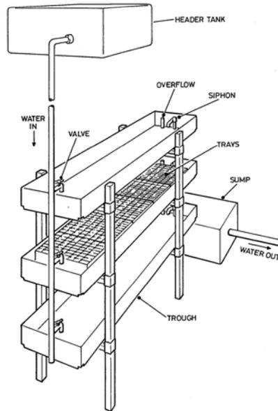
Figure 1: Siphon and overflow arrangements in a trough on-growing system
