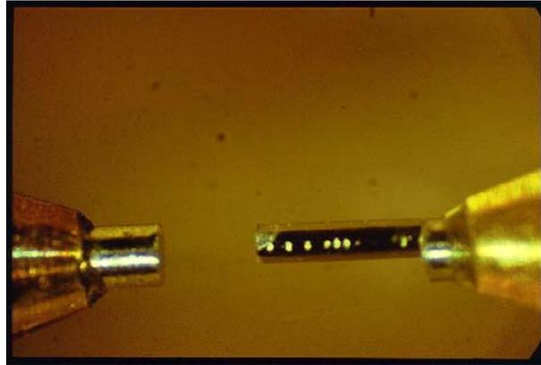
Plate 33: 1 mm long coded wire tag showing part of the binary-coded data sequence etched on its surface
