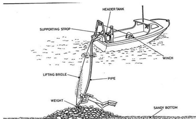
Figure 7: Diagram of the pipe release system
