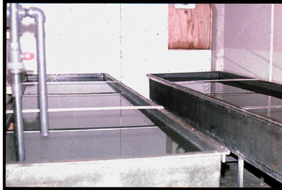
Plate 2: GRP tanks used for housing broodstock
