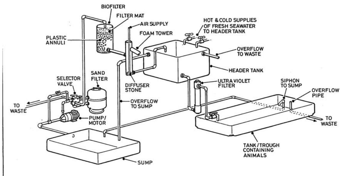
Figure 2: Diagrammatic representation of a filtration system
