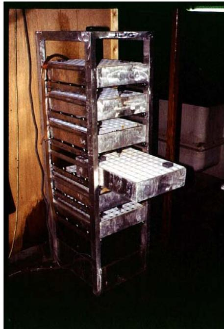
Plate 9: Experimental vertical stacking on-growing system
