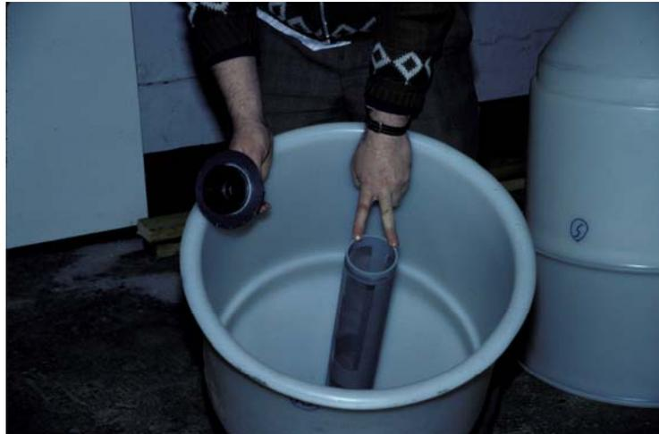
Plate 4: Diffuser and screen for larval tub
