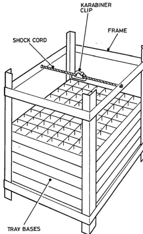
Figure 5: Arrangement of stack for release
