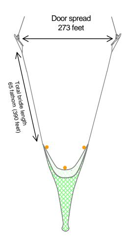
The skipper's target door spread is 60% of his total bridle length. 60% of 390 feet is 234 feet.
