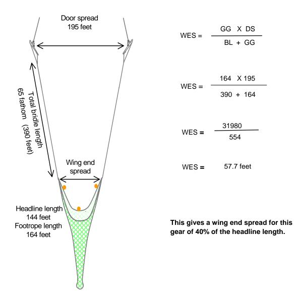
If this calculation is to be used in a twin rig set up the overall door spread must be halved. Each net and its respective bridles can be treated as a single trawl for this calculation. In comparison with wing end spread measurements from electronic sensors during sea trials this calculation gives respectable results. However, in some situations (ie. very long net and short bridles) the results may be distorted and unreliable.
