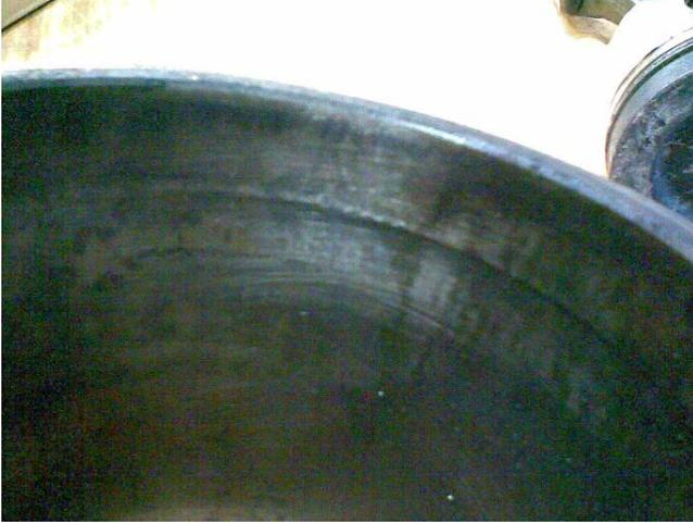
**Figure 1** Excessive wear: ring landing area
