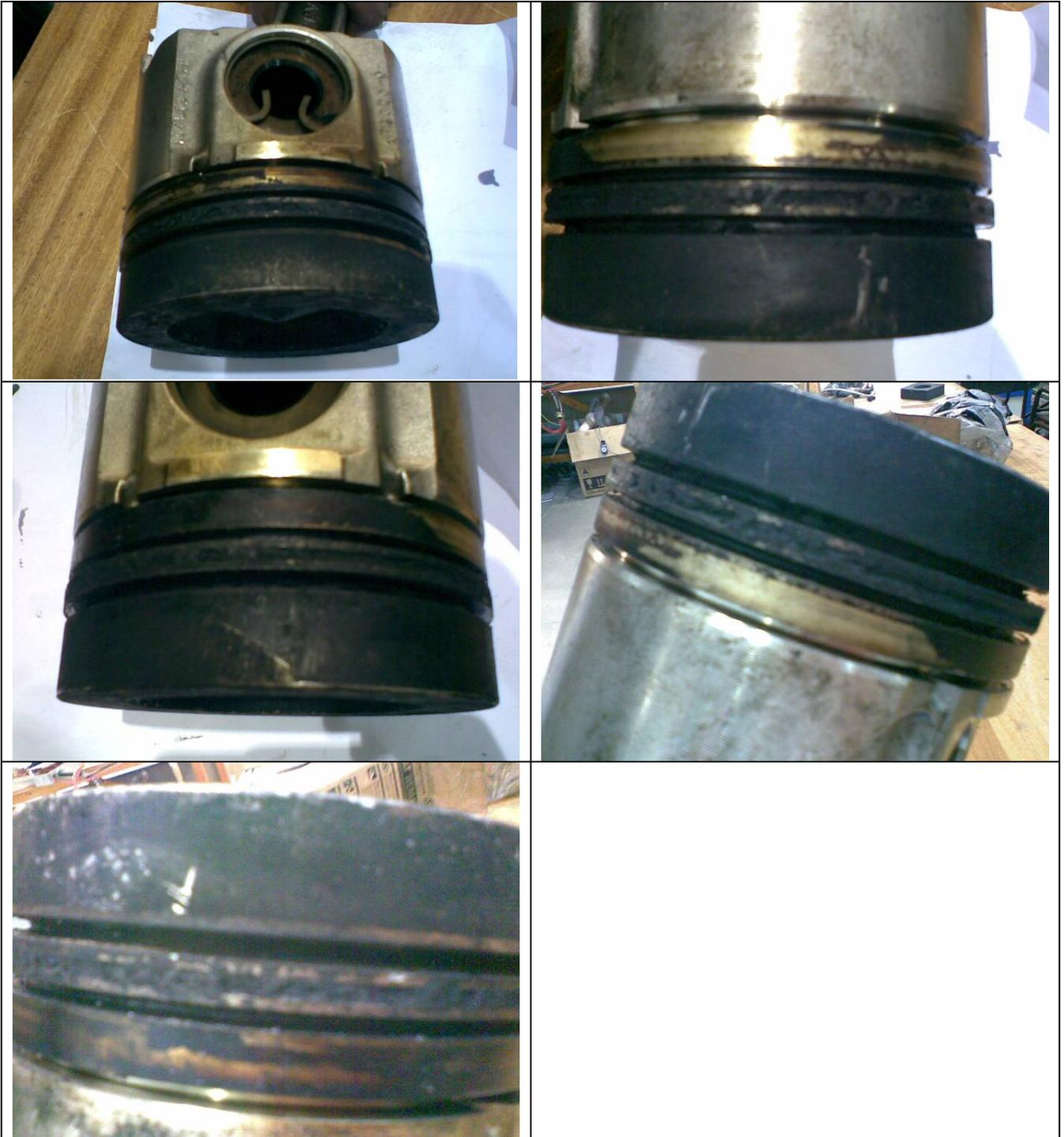
**Figure 3** Fingerprints for excessive blow by- possibly due to excessive wear of rings and liner at the ring landing area, hard carbon build-up between top and bottom ring
