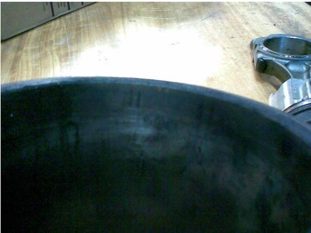
**Figure 4** Excessive carbon build-up
