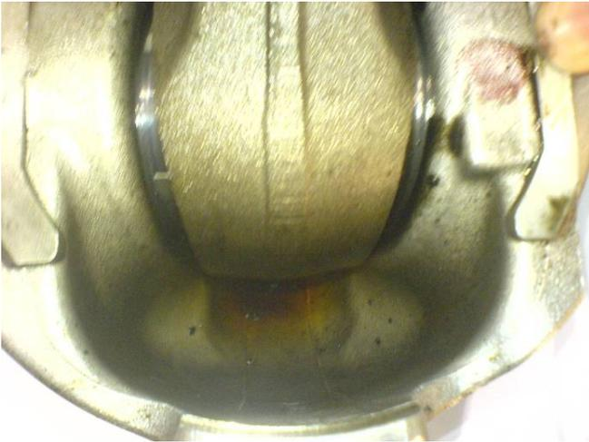
**Figure 5 Fingerprint for Overheating: under the piston crown**
