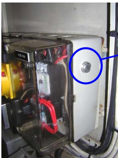
Temperature data logger fixed to switch box in engine room to capture ambient temperature (4). ALL loggers have been set to capture the temperature at 90 minute intervals. Each logger will hold approximately 25 days worth of data.
