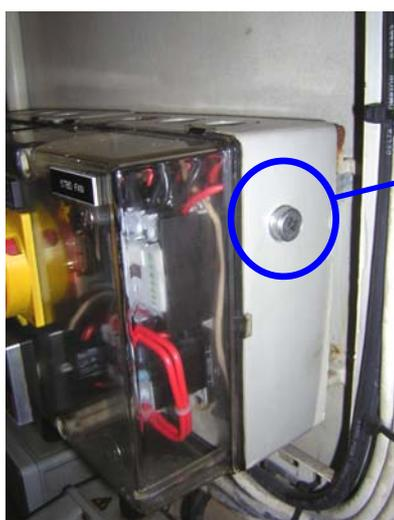
Temperature data logger fixed to switch box in engine room to capture ambient temperature (4). Loggers were set to capture the temperature at 60 minute intervals. Each logger holds approximately 5 months worth of data.
