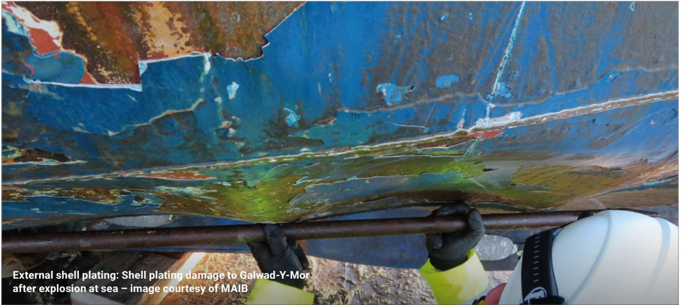
External shell plating: Shell plating damage to Galwad-Y-Mor after explosion at sea – image courtesy of MAIB
