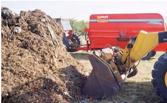
*Figure 12 – Photograph of Mixed Sea-food and Green-Waste being discharged from the Mixing Machine*
