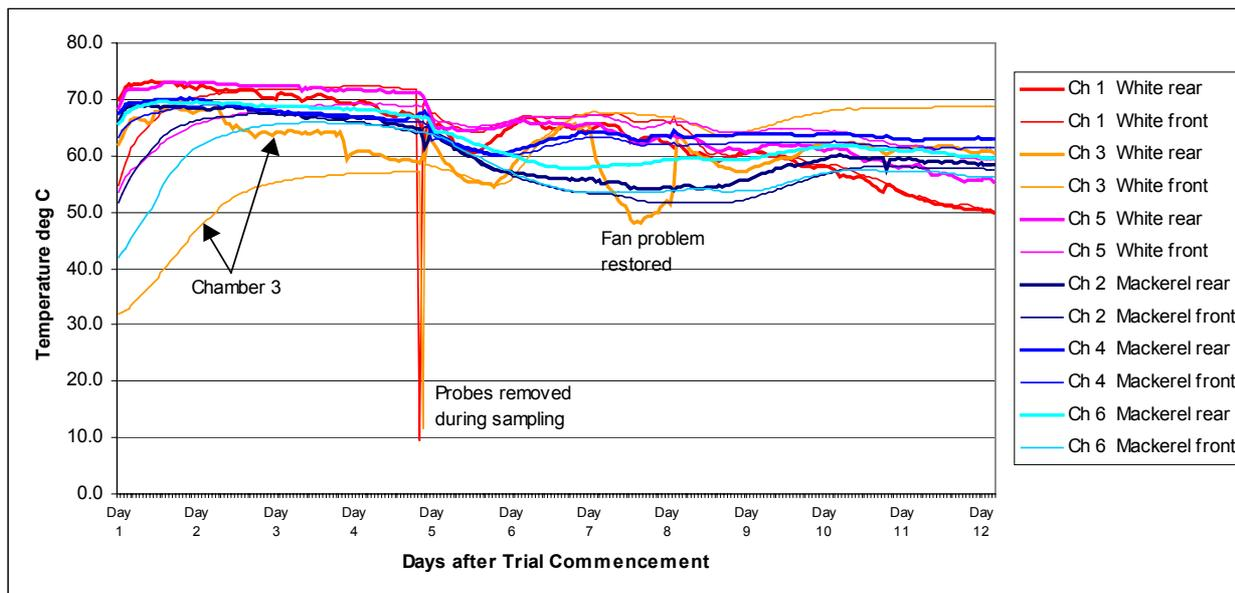
The effect of these temperature variations in Chamber 3 were borne out in the pathogen sampling and testing, where in Table 6 it can be seen that at day 4 there were still pathogens present in Chamber 3 where-as they were destroyed in all other samples.
