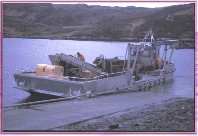
An example of a modern boat designed to service longlines used for rope-mussel cultivation
