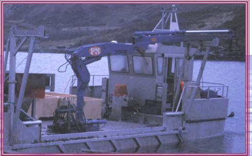
Cranes or lifting arms can be mounted on service rafts or boats
