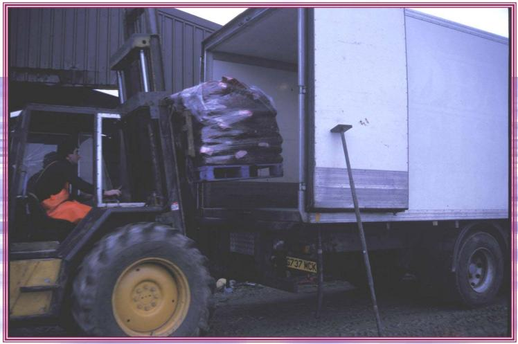
Using a forklift truck to load palletised mussels in to a chilled transport trailer
